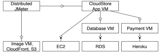
Fig. 2. CloudStore deployed on AWS.
